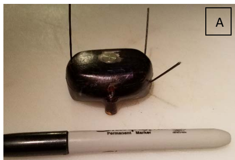
Figure 1. A) Fastloc GPS-LIMPET tag in the SPLASH10-F-333B configuration. B) GPS-LIMPET deployed on an adult male Cuvier's beaked whale (ZcTag053).
